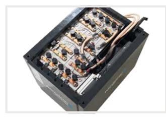
In this 48V example, the complete battery pack is assembled. The BPU is installed and the cell monitoring wire to each of the 15 cells in series are mounted for cell voltage sensing and balancing.
